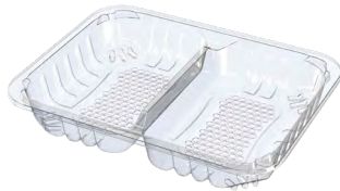
Holzorb Recyclable tray technology that uses grooves and pockets to trap liquid, eliminating the need for non-recyclable absorbent pads
