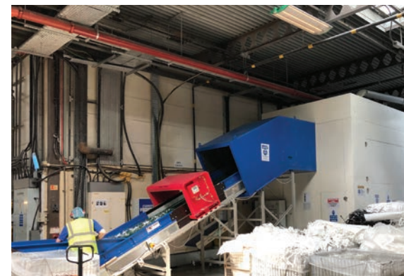
Through years of process engineering and investments in manufacturing, thermoforming operations focus on optimizing the use of raw material, capturing engineered waste so it can be reused. This reduces our reliance on virgin content.
