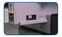
Start by sliding the tower partially or fully out of base (do NOT place on side or tip upside down, keep the tower upright).
