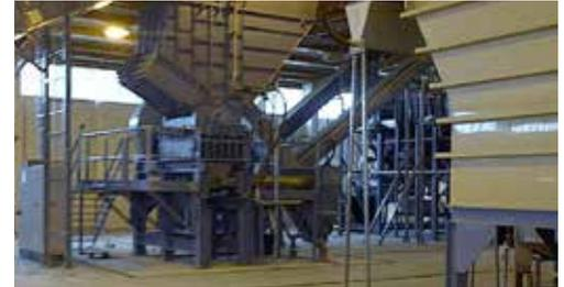
To assist customers looking for a sustainable solution to their packaging needs, a 100,000 sq. ft state-of-art recycling facility is operated in Shawano, Wisconsin - to sort, shred, wash and pelletize post-consumer film scrap. **This process redirects over 13 million lbs. of post-consumer film scrap from the landfills back into reusable industrial packaging.**
